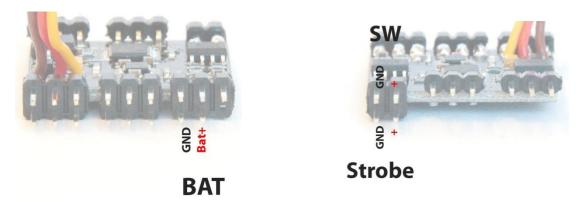
Connect battery to **Bat** connector. Connect headlight LEDs to switch output connector **Sw**. Connect strobe LEDs to **Strobe** connector.
