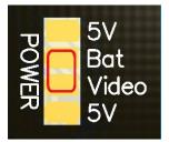
Battery will power Video connectors and Switch output.
